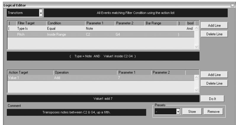
Figure C.1 The Logical Editor used to transpose notes between C2 and G4 up a fifth
